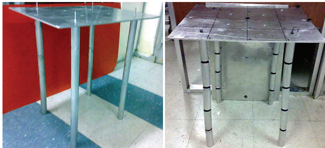
Fig. 18. The simulation platform model: (a) with plain legs, (b) with periodic legs.
